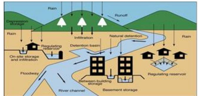
Picture 1- Illustration of Integrated Drainage System or Known as Comprehensive Flood Control Map
